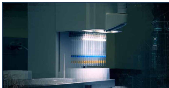
Integra Viaflo 96 with DPX WAX/RP Tips
