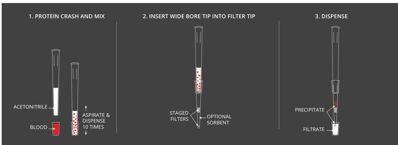
Figure 2. Schematic of the DPX Tip-On-Tip method for automated protein crash of blood.
