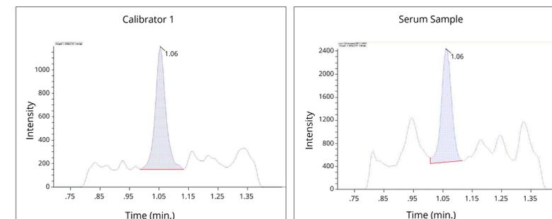
Figure 4. Chromatogram for a calibrator at the Limit Of Quantitation (LOQ), 0.02 ng/mL.
