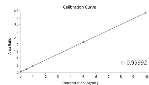
Figure 3. Representative example of a six-point calibration plot calculated from this Tip-on-Tip Method (r = 0.99992)
