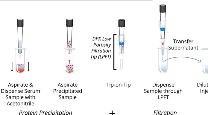
Figure 2. DPX ToT method which takes <5 minutes to perform. Sample preparation was performed on a MICROLAB® NIMBUS96 open layout liquid handler.
