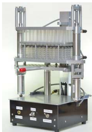
Figure 1. DPX 5 mL Pneumatic Extractor is a syringe device that operates under gas to create positive and negative pressure to aspirate and dispense solutions in and out of 5 mL tips
