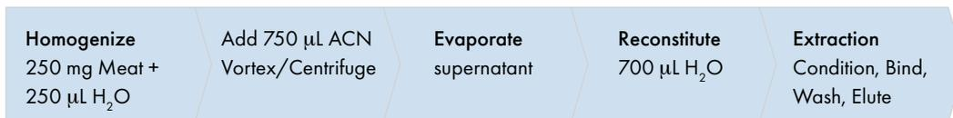
Figure 1. Sample pretreatment and Dispersive Pipette XTRaction protocol. After elution the solution is solvent evaporated and reconstituted in 100 µL of 5% methanol, 0.1% formic acid in water
