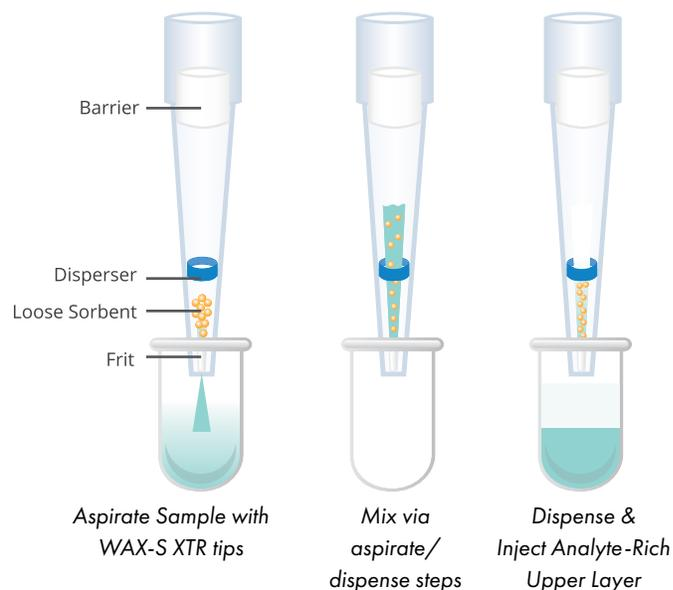
Figure 2. Visual representation of Dispersive Pipette XTRaction method that uses salt-assisted liquid-liquid extraction (SALLE) in addition to SPE. Note the analyte-rich acetonitrile upper layer in the final solution, now ready for analysis.
