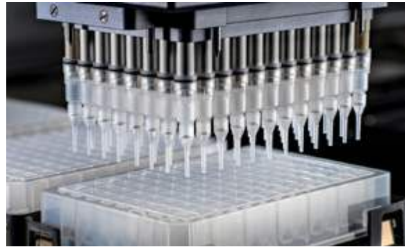
Robot head directly engages the MPX devices after the vacuum step. Elution is dispensed directly into the final well plate.
