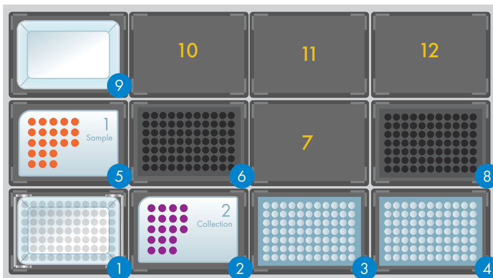
Figure 3. Deck layout for SEC workflow described above on a Hamilton Microlab Nimbus.
