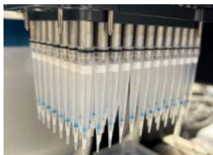
Figure 1. The deck layout used for the Hamilton NIMBUS 96 automated liquid handler (ALH) and a photograph of 96 HLB DPX Tips.
