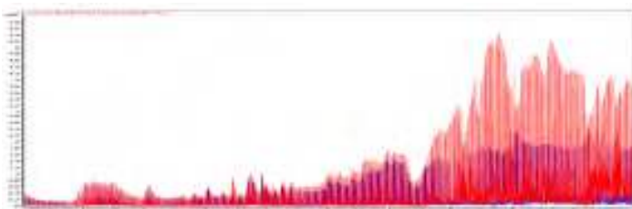
Figure 3. Chromatogram showing the reduced background from an extracted protein crash (red) compared to using a protein crash in conjunction with DPX Technologies' SEC Tips (blue).
